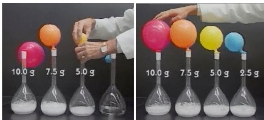
Figure -10. Specified masses of \text{NaHCO}_3(\text{s}) are added to 100 mL samples of vinegar resulting in the reaction, \text{NaHCO}_3(\text{s}) + \text{CH}_3\text{COOH}(\text{aq}) \rightarrow \text{NaCH}_3\text{COO}(\text{aq}) + \text{H}_2\text{O} + \text{CO}_2(\text{g}) .
